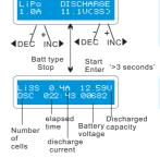
The value of discharge current on the left cannot exceed 1C, and the value on the right cannot be under the voltage recommended by the manufacturer to avoid deep discharging. Press STAR/ENTER for more than 3 seconds to start charging.
