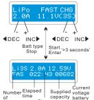
Charging current will become lower when it progress to the end of charging. A specific CV process will be reduced to end the charging process earlier. In fact, the charging current will goes to 1/5 when the charging process comes to 1/10. Charging capacity will be a little smaller than normal charging, but charging time will be shortened accordingly.
